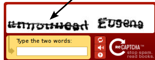
Figure 1: reCAPTCHA digitization example. OCR software reads the circled word as “announcac1,” but with low confidence. This word is then extracted and presented as a CAPTCHA challenge to users, who type in the correct spelling: “announced.”
