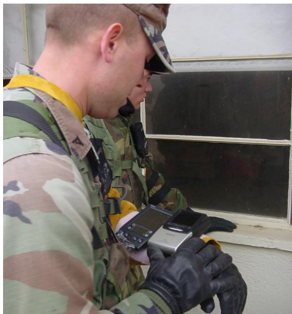
Fig. 5. Operator wearing prototype user interface. Commands can be issued via the PDA while the LCD monitor is used to view video transmitted from a Scout.
