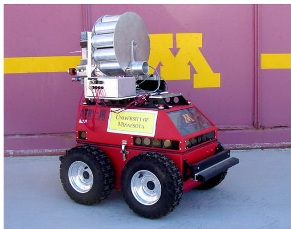
Fig. 2. The Ranger with a custom-built magazine for ten Scouts.
